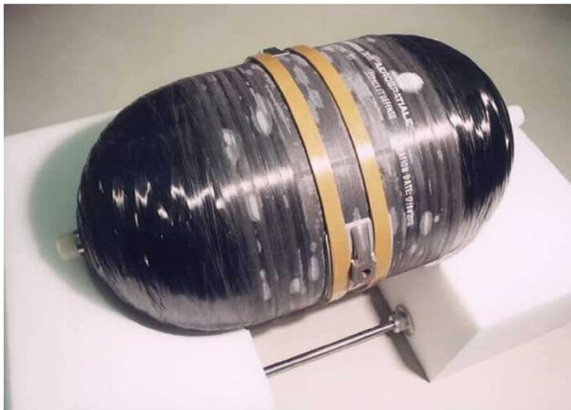
**Fig.7: EADS Carbon vessel with Titanium Liner ( 80 liters- 17,7 Kg )-**
