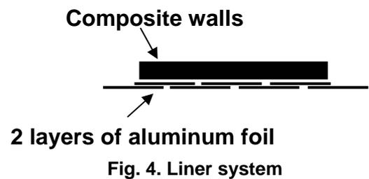
The external tank is equipped with only one metallic polar bosses (bonded closure on the other one). The interface between composite walls, the liner system and the bosses is one of the major singularities. One of the best concepts is the packing gland-type boss with reinforced domes. Three of the main metal selection criteria are the chemical liquid oxygen compatibility, mechanical characteristics at 90K and the thermal contraction at 90K.
