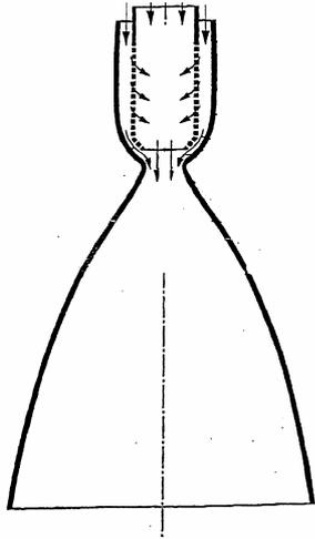
**Fig.5: Transpiration cooled Chamber principle using PTAH-SOCAR [R6]**
