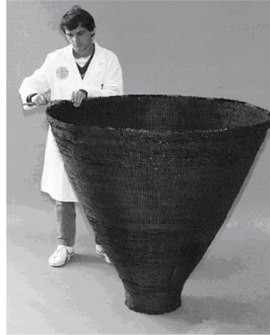
**Fig.6: One of the first large nozzle perform woven at EADS**
