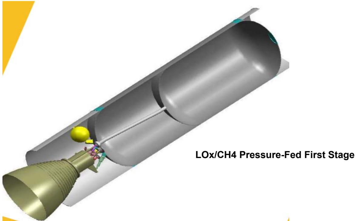
A pressure-fed liquid stage will be better than a turbopump one if with the same specific impulse( same combustion pressure), its structural index is better than a turbopump one.
