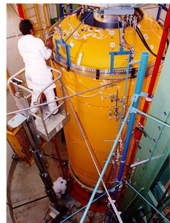
**Fig. 6.** Internal pressure test facility at EADS-LV
