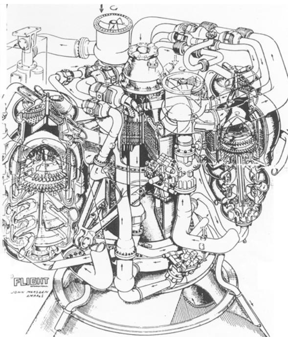
For Liquid stage an engine is costly due to the high cost of turbopumps(=30 to 50% of engine cost, the engine may represent 50% of stage cost) . Moreover, complexity equals loss of reliability.
