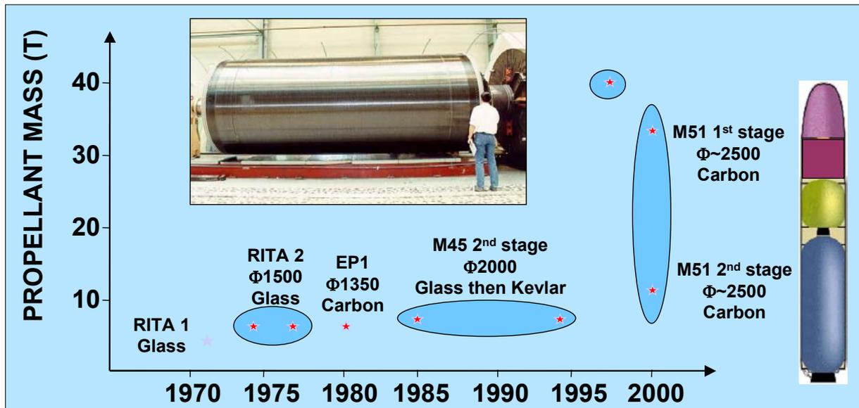
All of these developments and mass productions represent more than 600 manufactured motor cases and about 150 tons of filament wound composite combined mass from 1970 until today :
