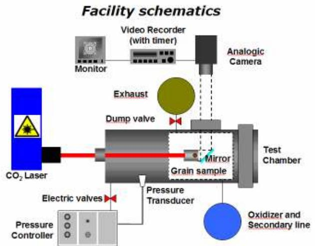
Fig. 4 Overall sketch of the hybrid test facility.
