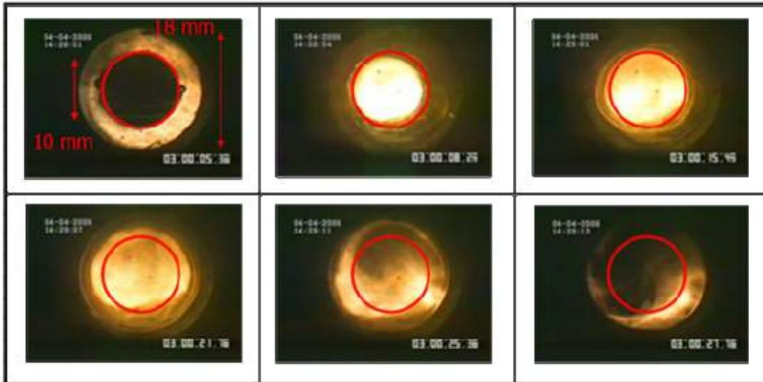
Figure 6: Video-recording frames of a typical burning test
