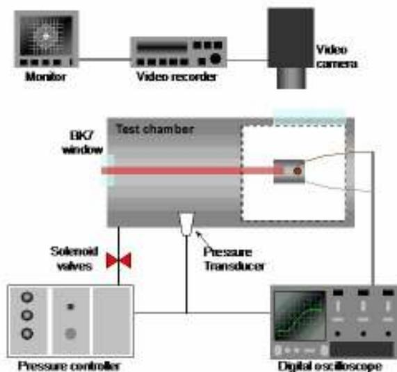
Figure 9: Schematic of the experimental set-up
