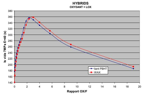
Fig 2 : Isv evolution vs O/F (Wax and HTPB)
