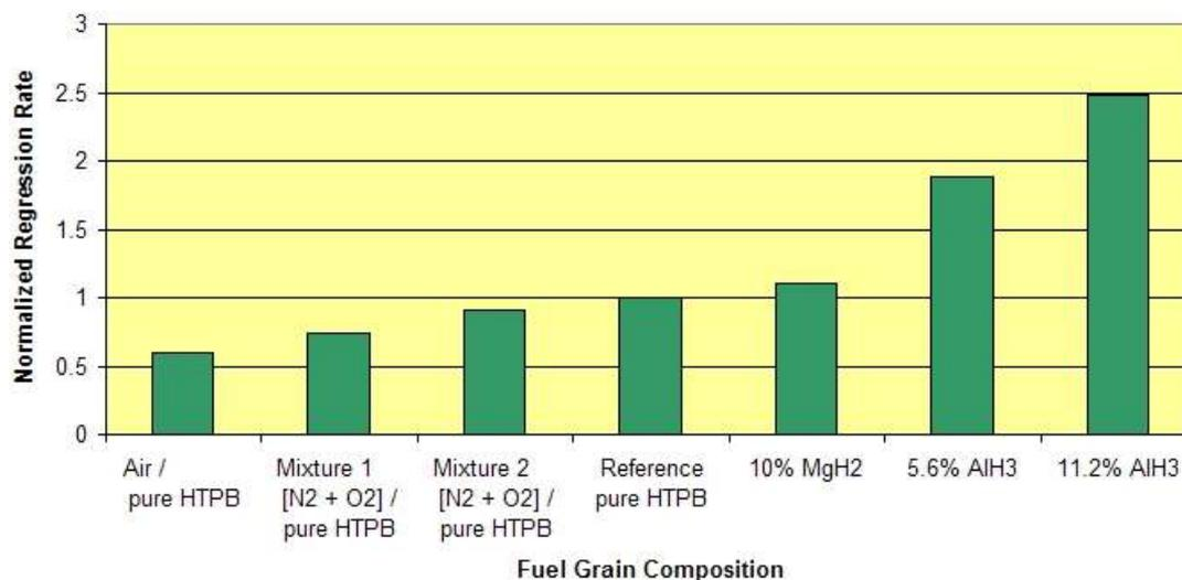
**Fig. 10: Effect of Hydrides on the regression Rate**
