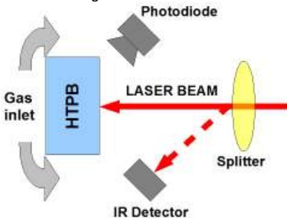
Figure 7: Setup for the ignition delay measurement
