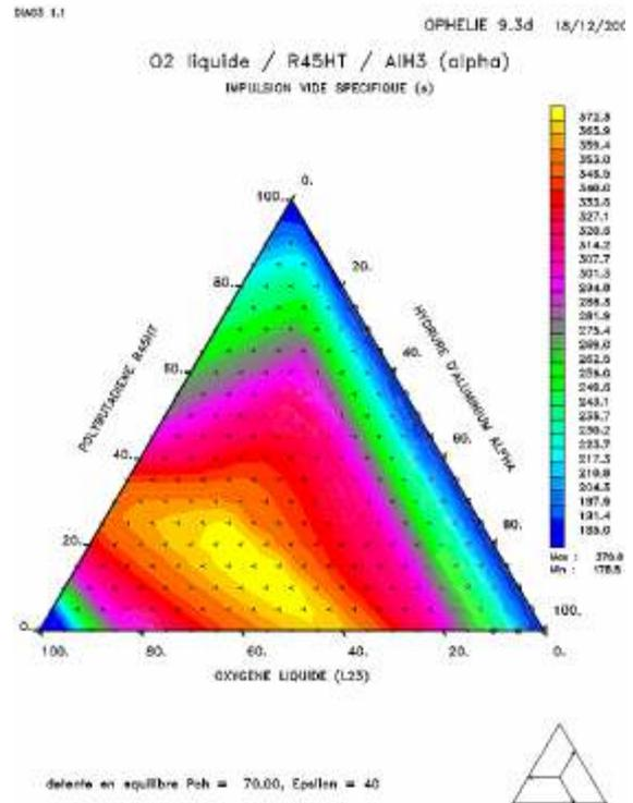
Fig.3: Ternary Diagram for HTPB/Alane/LOX
