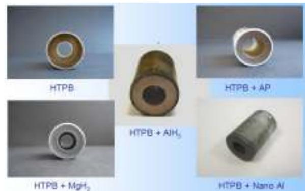
Fig. 5 Test samples
