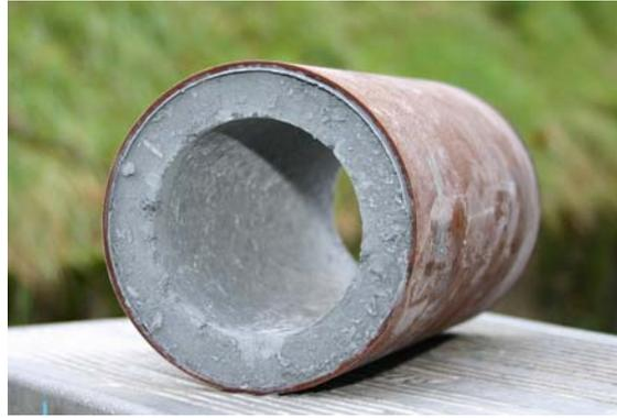
**Figure 9 – BATES grain after storage**
