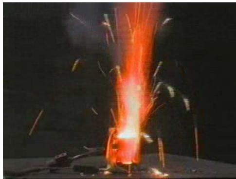
**Figure 8 - Combustion of Mini-BATES grain at atmospheric pressure**
