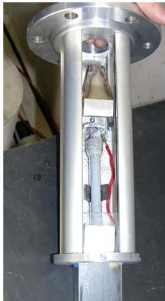
**Figure 6 - Experimental pipe filled with refrigerated solid propellant (ICARE Picture)**
